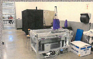
Immersion testing tank
